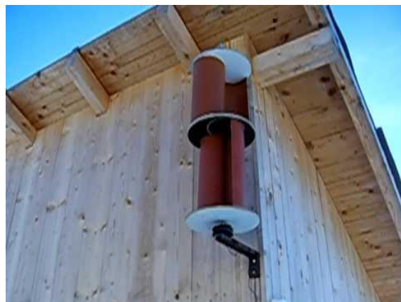
Picture 9. Savonius low power turbine
